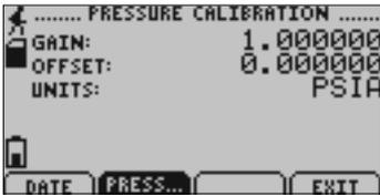
*Displays calibration information for pressure channel.*
