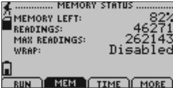
*Displays information about the device's memory capabilities including percent of memory available (memory left), number of readings taken so far (readings), max number of readings (max readings), and wrap status.*
