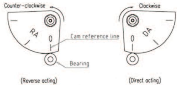
**Attaching Procedure of Opening Degree Indication Plate**
