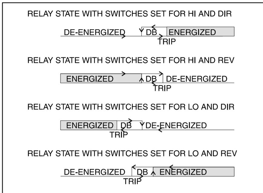
Using the figure below, set up the switches on SW2 for Alarm A and Alarm B. For dual alarm relays triggered by Alarm A, set switch 5 to DUAL. When switch 5 is set to DUAL (on), switches 6 and 7 have no effect.
