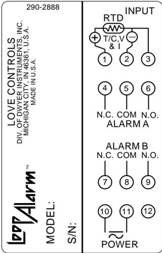
For SC1090, power is 85 to 265 Vdc/Vac 50 to 400 Hz.
