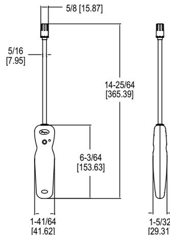
The **Model RP3 Wireless Thermo-Hygrometer Probe** measures relative humidity, temperature, dew point, and wet bulb temperatures when combined with the UHH4 or newer universal handheld device, or your own mobile device. In order to protect the sensor in higher air flow ducts, each probe comes with a membrane filter. Factory calibrated replacement humidity sensors can plug directly into the probe without requiring additional calibration.
