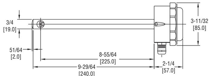
The Series AVUB Air Velocity Transmitters from Dwyer Instruments are suitable for measuring air velocity within a duct and giving a 0 to 10 V linear output. A typical application would be in a VAV air conditioning system.
