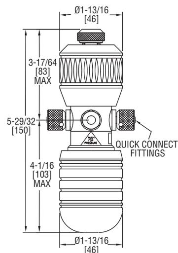
The Model HP Hand Pump provides a dual source of pneumatic pressure and vacuum for verifying the calibration of pressure instrumentation. Pump can generate pressures up to 45 psi (3 bar) and vacuum to -27" Hg (-910 mbar). The compact pump is designed for portability and single hand operation.
