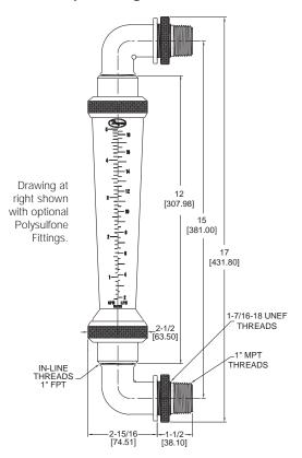
The Series UV In-Line Polysulfone Flowmeter measures the flow of water, air, and other compatible media at temperatures up to 212°F (100°C) and pressures up to 150 psi (10.34 bar). This flowmeter's highly corrosion-resistant materials suit it ideally for use with de-ionized water and ultra-pure applications, including food processing, medical equipment and reverse osmosis water systems.
