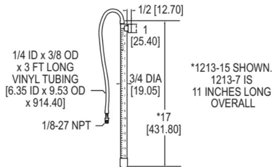
The **Series 1213 Gas Pressure Manometer** provides visual indication of pressure of natural gas up to 15 in w.c. Tap water is used as the sensing media and a magnetic clip provides temporary or permanent mounting. The 1213 is made of a durable plastic for years of trouble-free service, and includes 3' of vinyl tubing and 1/8" nylon male NPT to barb fitting.
